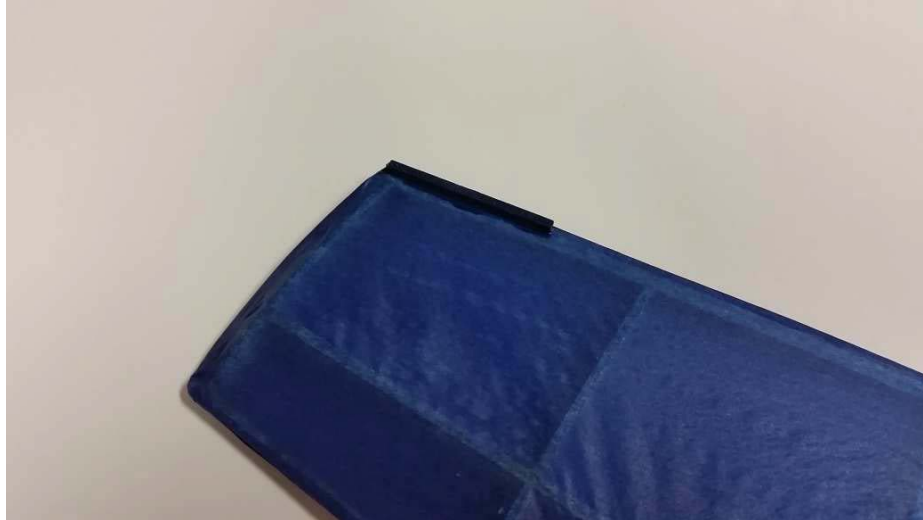
Gurney Flap Glued to Top Side of Trailing Edge of Right Wing Section
