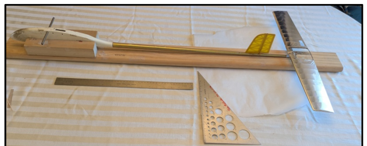
In the jig—aligning pod, boom and stab
