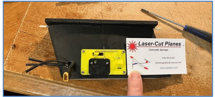
Button, vertical-axis servo, switch, mousetrap. Business card for size comparison. I'm working on making it smaller still.
